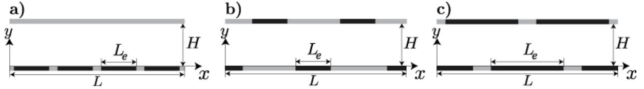
Figure 1: The modeling domain. The black and grey boxes represent the electrodes and dielectric surfaces, respectively.
