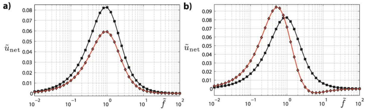
Figure 4: The dependence of the flow rate on the AC field frequency. The left plot shows the comparison of the variant 1a) (black line) and 1b) (red line) with the same length of electrodes. The right plot show the comparison of variant 1a) (black line) at  $L_e = 0.2$  and variant 1c) at  $L_e = 0.4$ .
