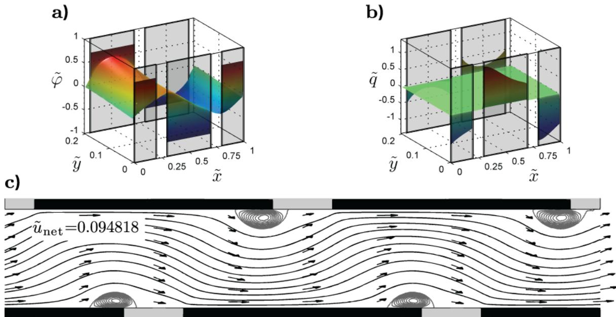
Figure 2: Profiles of system quantities at the optimal frequency and zero back-pressure: a) The electric potential; b) the electric charge density; the flow velocity. AC amplitude: 25.7 mV,  $L = 100$  Debye lengths.
