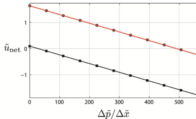
Figure 3: The dependence of the flow rate on the applied back-pressure gradient at the amplitude  $A = 1$  (black line) and  $A = 10$  (red line).
