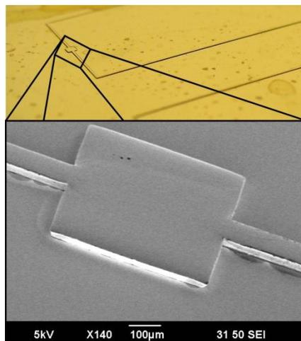
**Figure 1. Optical microscope and SEM images of micro structures on copper-gold stamp**
