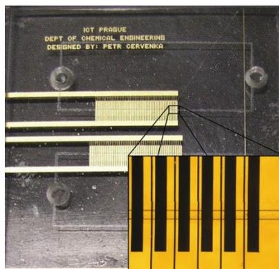
**Figure 2. AC electroosmotic pump, detail on the PMMA microchannel across the microelectrode array**
