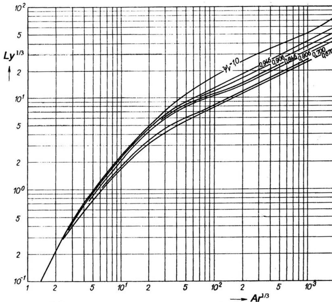
Fig. 7-1 Dependency of  $Ly^{1/3}$  ( $Ar^{1/3}$ ,  $\psi_V$ ) for the sedimentation of spherical and non-spherical particles in the transitional and turbulent regions. The parameters of the curves is the sphericity  $\psi_V$
