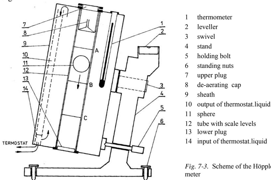
Fig. 7-3. Scheme of the Höppler viscosity meter
