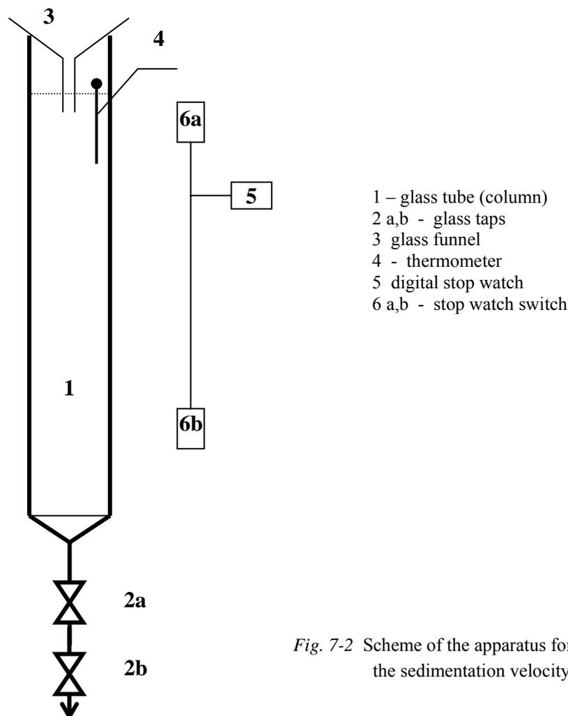
Fig. 7-2 Scheme of the apparatus for measuring the sedimentation velocity of particles
