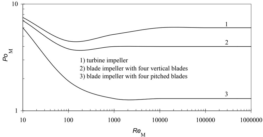
Fig. 9-2 Dependence of the power number on Reynolds number for different kinds of impellers in a baffled vessel ( $D/d = 3$ ;  $H/d = 3$ ;  $H_2/d = 1$ ;  $n_b = 4$ )
