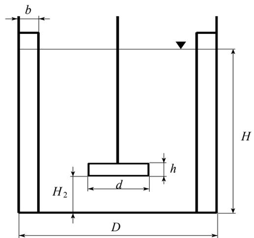
Fig. 9-1 Scheme of a mixing apparatus
