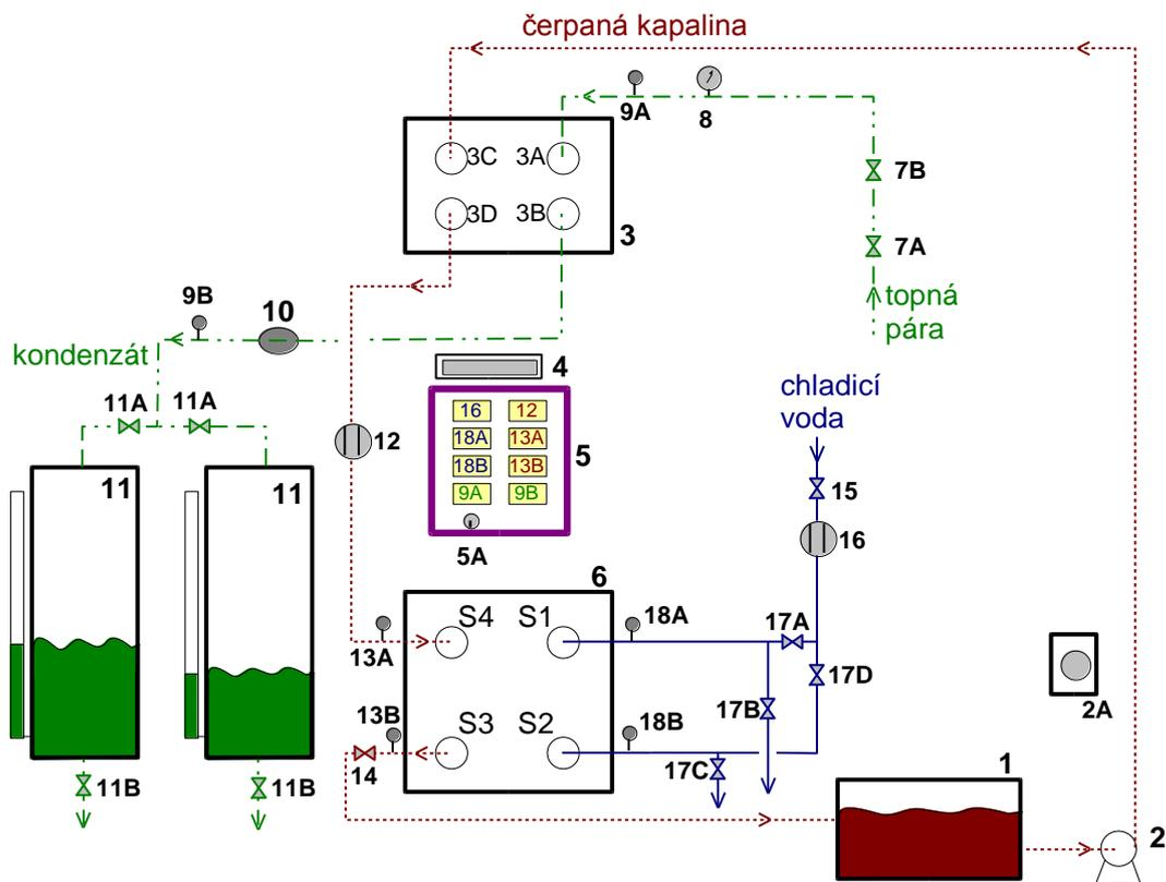
Fig. 11-4 Heat exchanger station T1 layout.
