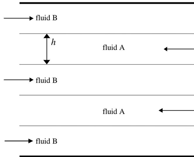
Fig. 11-3 Scheme of the plate heat exchanger
