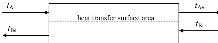
Fig. 11-2 Counter-current streams arrangement
