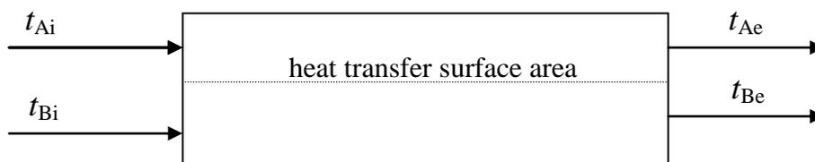
Fig. 11-1 Parallel streams arrangement
