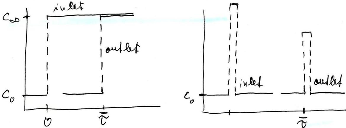
Plug flow is a basic flow pattern assumed in the flow through tubes and packed beds. In reality, it can be disturbed by **axial dispersion** –  $F(\tau)$  then becomes flatter and  $E(\tau)$  broadens.
