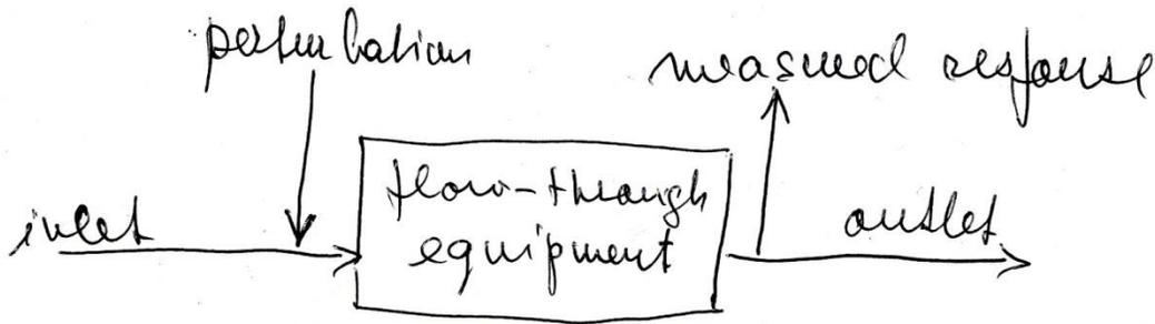
Typically, the perturbation is realized by introducing a **tracer** – a soluble component whose concentration is measured at the outlet. Particles (molecules) of the tracer are carried by fluid particles and represent their occurrence in the equipment and at the outlet.
